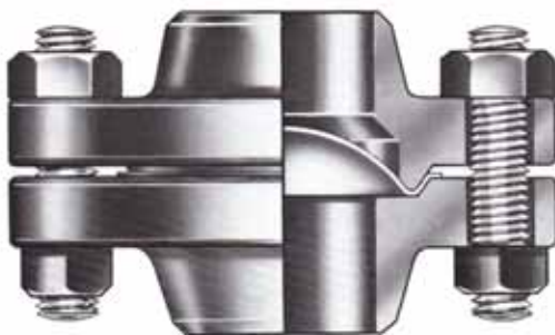
Figure 30: Bolted type fitting with welding hub flanges.
