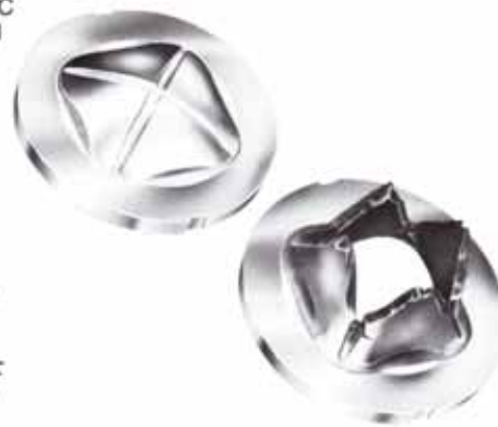
Figure 25: High pressure disks used in quick opening valve assembly, before and after rupture.
