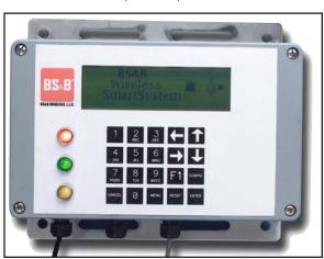
to activate its internal switch to handle up to 1/2 Amp of external power. This feature can be used for field annunciation (horn, lamp, etc.) or control purposes; higher currents can be accommodated using additional field hardware.
