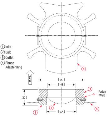
The proprietary shape of the Flange Adapter Ring ensures a well centered fit between typical companion flanges.
