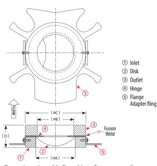
The proprietary shape of the Flange Adapter Ring ensures a well centered fit between typical companion flanges. Actual shape varies.
