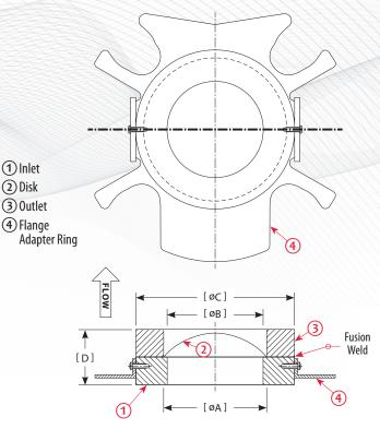
The proprietary shape of the Flange Adapter Ring ensures a well centered fit between typical companion flanges. Actual shape varies according to nominal size.
