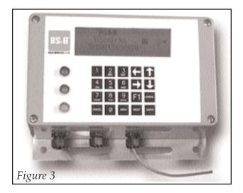
Use of a 12-bit A/D converter means the resolution of data within SmartDisk/SmartSystem is excellent. The overall accuracy of information generated through this wireless system is determined by:
