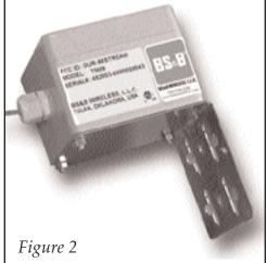
\*Note: The use of a Planar Omni-Directional antenna avoids the need to perfectly align each DTM/ATM with its system RTM. Many RF signals will reach their destination by reflection making "line of sight" unnecessary. Use the 'site survey kit' or the DMM/DM4 "received signal strength" feature to determine when each DTM or ATM is well aligned for RF service.
